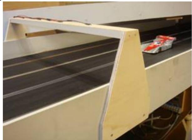
Mount sensors in the bridge and light sources from the track underside. Even though a 5 mm hole makes a good tight fit with the LED's, you can use glue or duct tape to lock the LED's in place.
