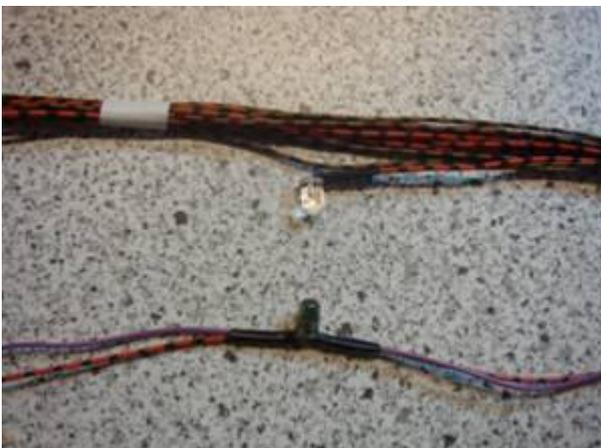
The IR sensors consist of a light source (The bottom “smoke” colour LED in the picture), which emits IR (infra red) light, and an IR-sensor (clear colour LED), which changes conductivity when subjected to IR-light.
